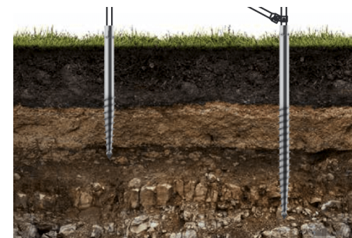
Fig.9 Illustration de pieux vissés (source Bayo's)
