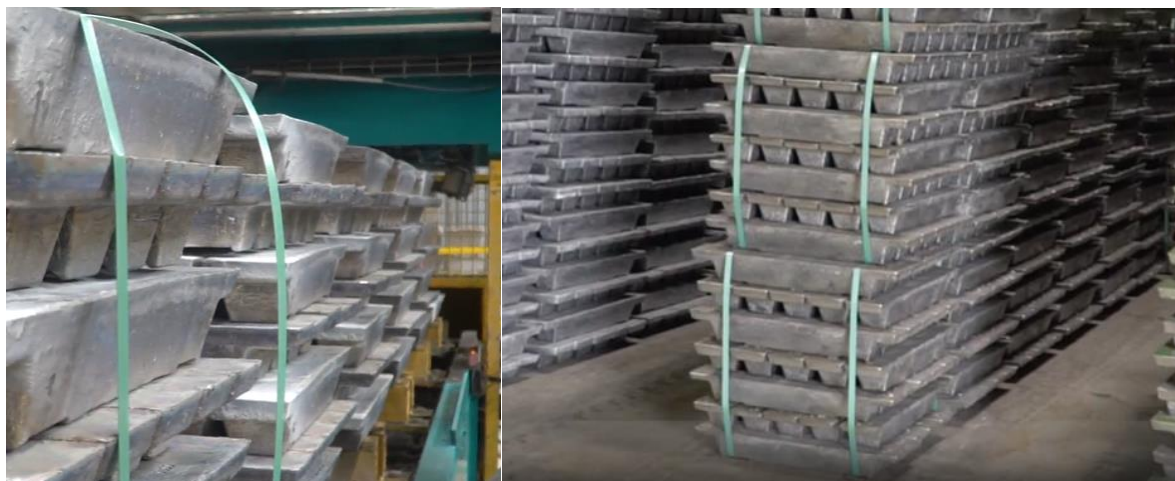
Figure 22 : Stockage et cerclage des lingots de plomb (source international lead association)
