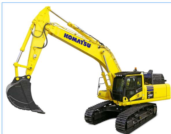
Figure 97 : Exemple de pelle 49t Komatsu PC490/LC-11
