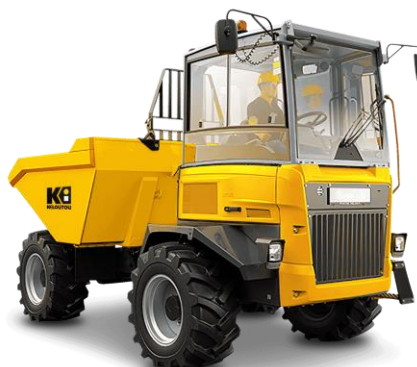
Figure 62: Exemple dumper 9T capacité
