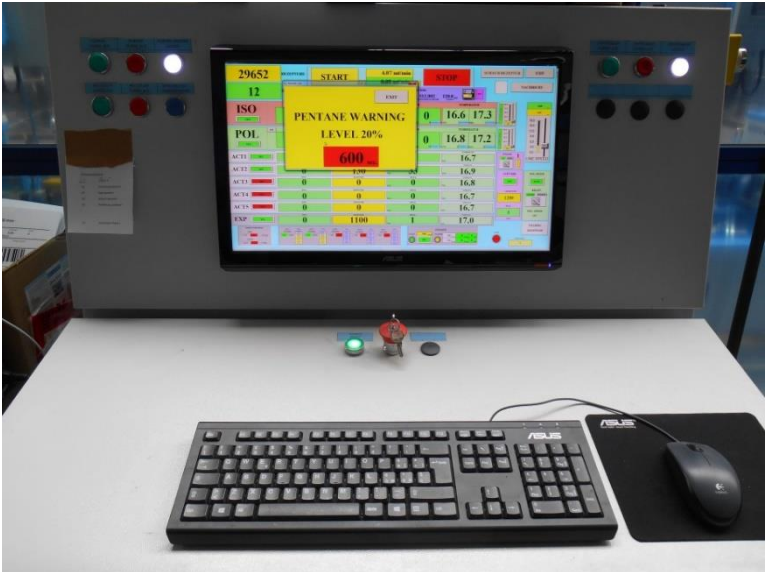
Picture of the 20% level detection warning screen available from the main computer supervisor, with the down counting seconds remaining before the production automatically stopped.
