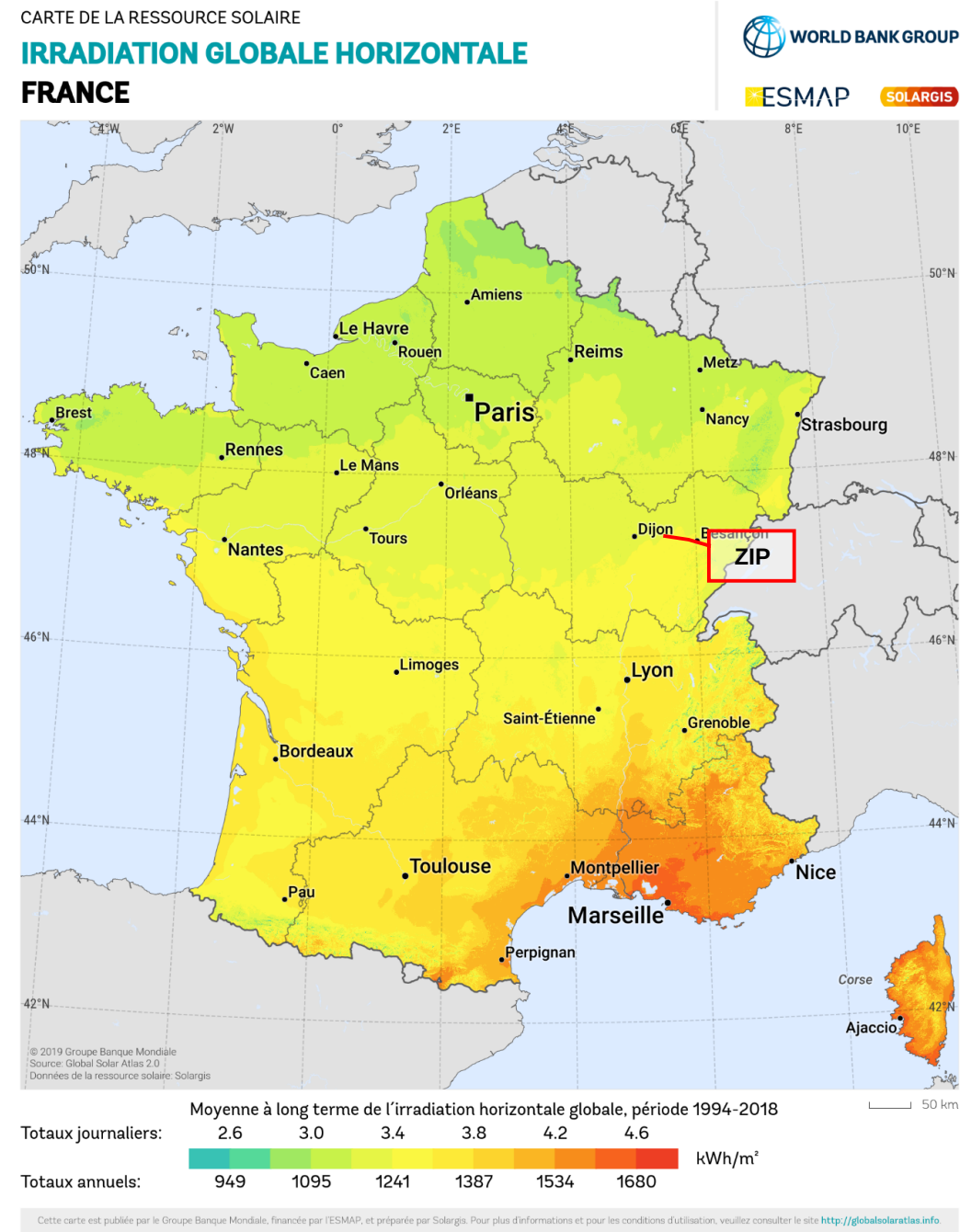
Figure 3-21 Irradiation globale annuelle de la France (source : Solargis)
