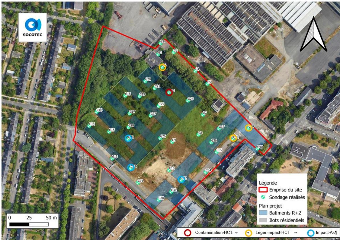
FIGURE 7 : SYNTHESE CARTOGRAPHIQUE DES CONTAMINATIONS SUR LES SOLS (SOURCE : DIAGNOSTIC COMPLEMENTAIRE JUILLET 2024)
