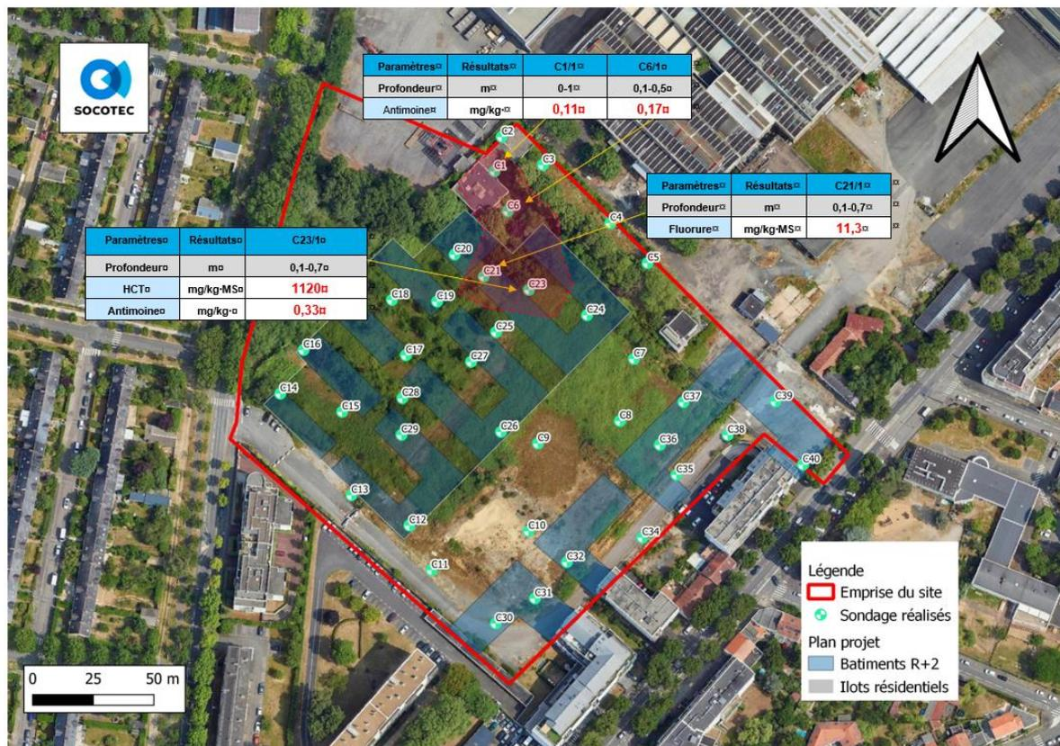
FIGURE 8 : SYNTHESE CARTOGRAPHIQUE – ADMISSIBILITE DES DEBLAIS EN ISDI (SOURCE : DIAGNOSTIC COMPLEMENTAIRE JUILLET 2024)
